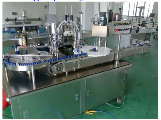
**Usage:** This machine is mainly suitable for automatic filling, stoppering and screw capping of electronic cigarette liquid, eye drops, nail polish, eye shadow, essential oil, with filling volume less then 50 ml.
