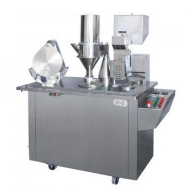
5.It has an infinite variable speed of filling table with independent power and fixed point filling that results in accurate dosage.
